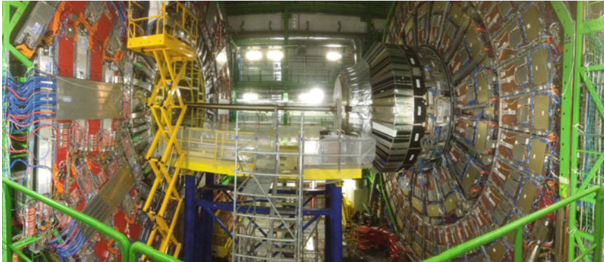
Fig. 3.9 Panoramic picture of the CMS detector, taken in January 2017. During this shutdown period, the detector was opened in order to check and repair some components; one can see the beam pipe in the middle, and on the RHS (LHS) the forward (barrel) parts of the detector
