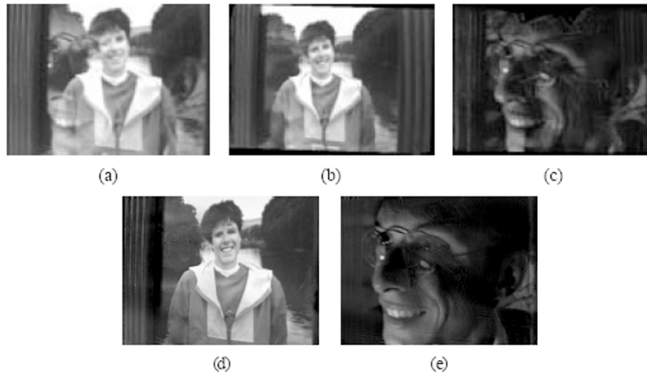
Figure 9.16 Light reflecting off the transparent glass of a picture frame: (a) first image from the input sequence; (b) dominant motion layer min-composite ; (c) secondary motion residual layer max-composite ; (d–e) final estimated picture and reflection layers. The original images are from Black and Anandan (1996), while the separated layers are from Szeliski, Avidan, and Anandan (2000) © 2000 IEEE.
