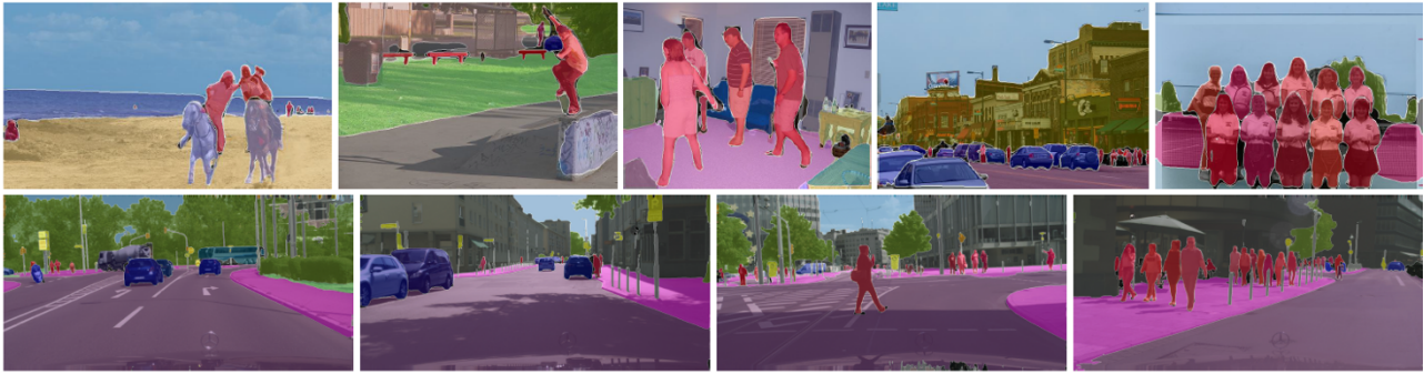
Figure 6.38 Panoptic segmentation results produced using a Panoptic Feature Pyramid Network (Kirillov, Girshick et al. 2019) © 2019 IEEE.
