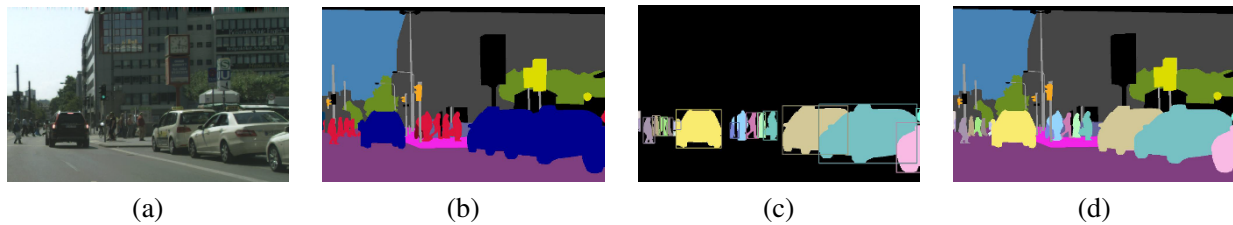
Figure 6.32 Examples of image segmentation (Kirillov, He et al. 2019) © 2019 IEEE: (a) original image; (b) semantic segmentation (per-pixel classification); (c) instance segmentation (delineate each object); (d) panoptic segmentation (label all things and stuff).
