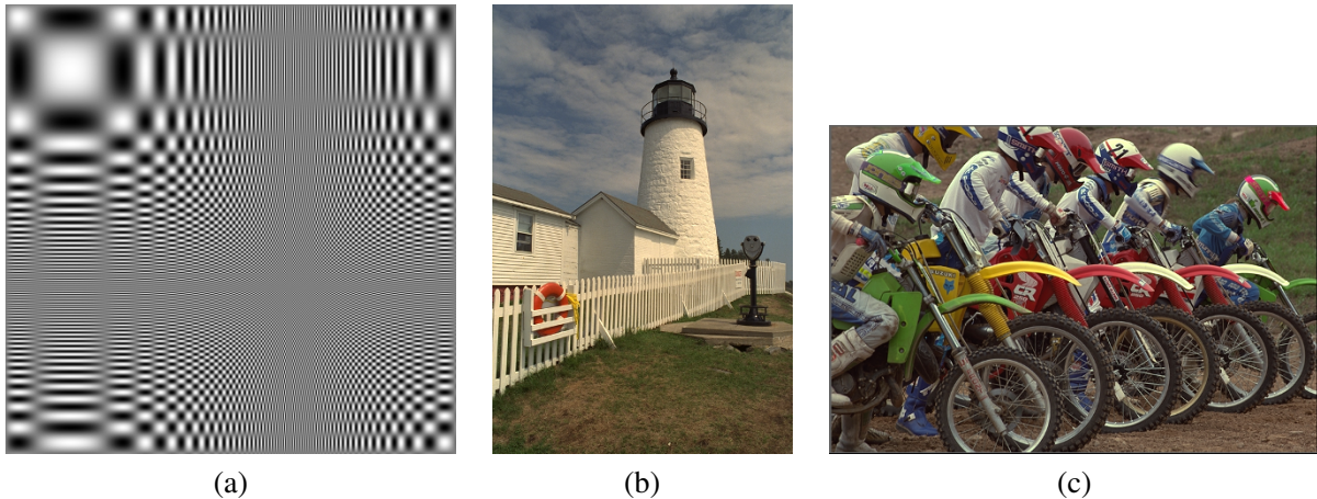
Figure 3.52 Sample images for testing the quality of resampling algorithms: (a) a synthetic chirp; (b) and (c) some high-frequency images from the image compression community.
