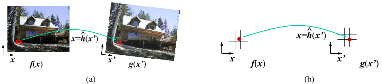
Figure 3.46 Inverse warping algorithm: (a) a pixel g(x') is sampled from its corresponding location x = \hat{h}(x') in image f(x) ; (b) detail of the source and destination pixel locations.
