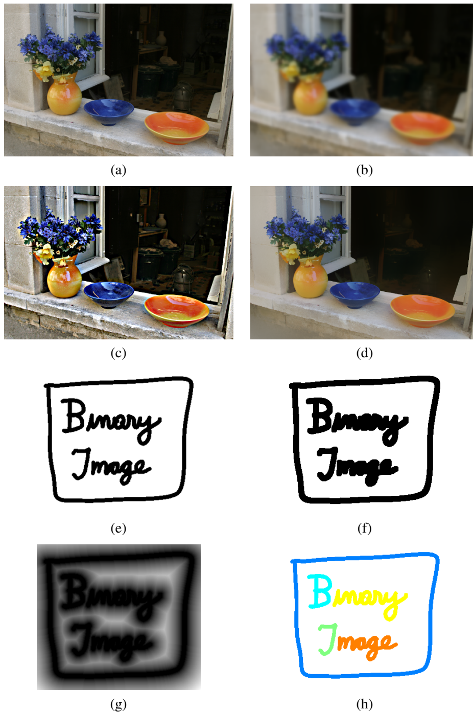
Figure 3.11 Some neighborhood operations: (a) original image; (b) blurred; (c) sharpened; (d) smoothed with edge-preserving filter; (e) binary image; (f) dilated; (g) distance transform; (h) connected components. For the dilation and connected components, black (ink) pixels are assumed to be active, i.e., to have a value of 1 in Equations (3.44–3.48).
