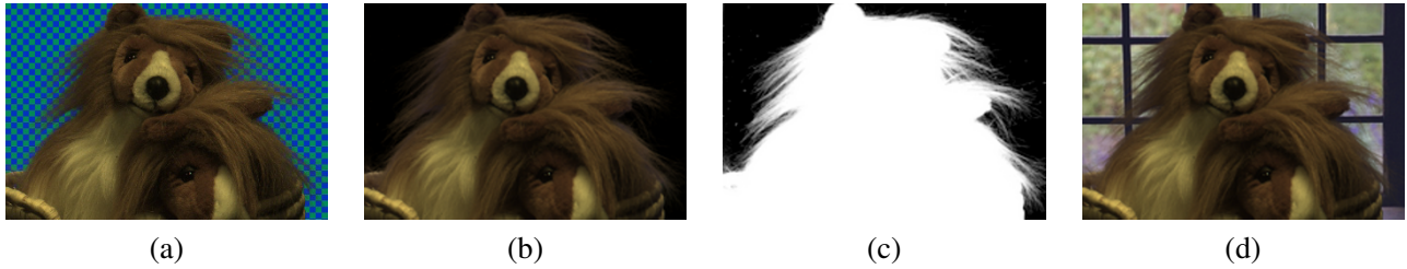
Figure 3.4 Image matting and compositing (Chuang, Curless et al. 2001) © 2001 IEEE: (a) source image; (b) extracted foreground object F ; (c) alpha matte \alpha shown in grayscale; (d) new composite C .
