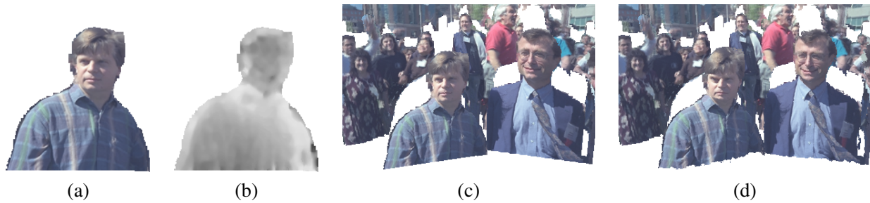
Figure 14.6 Sprites with depth (Shade, Gortler et al. 1998) © 1998 ACM: (a) alpha-matted color sprite; (b) corresponding relative depth or parallax; (c) rendering without relative depth; (d) rendering with depth (note the curved object boundaries).
