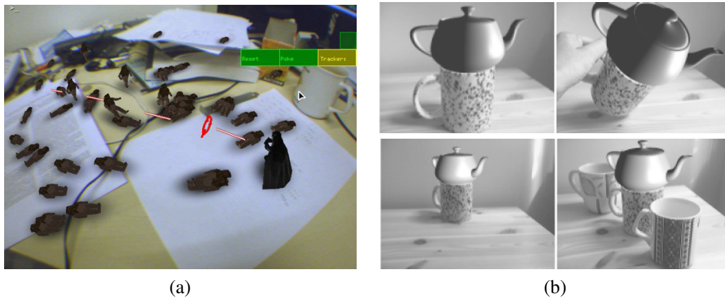
Figure 11.27 3D augmented reality: (a) Darth Vader and a horde of Ewoks battle it out on a table-top recovered using real-time, keyframe-based structure from motion (Klein and Murray 2007) © 2007 IEEE; (b) a virtual teapot is fixed to the top of a real-world coffee cup, whose pose is re-recognized at each time frame (Gordon and Lowe 2006) © 2007 Springer.
