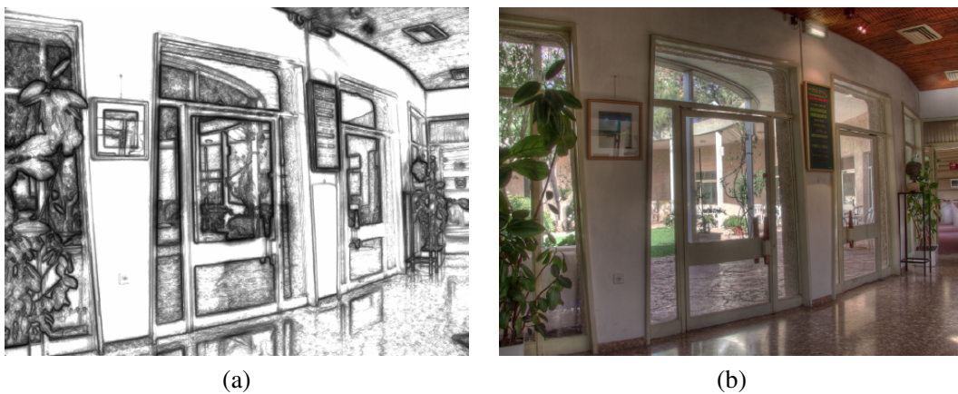
Figure 10.24 Gradient domain tone mapping (Fattal, Lischinski, and Werman 2002) © 2002 ACM: (a) attenuation map, with darker values corresponding to more attenuation; (b) final tone-mapped image.
