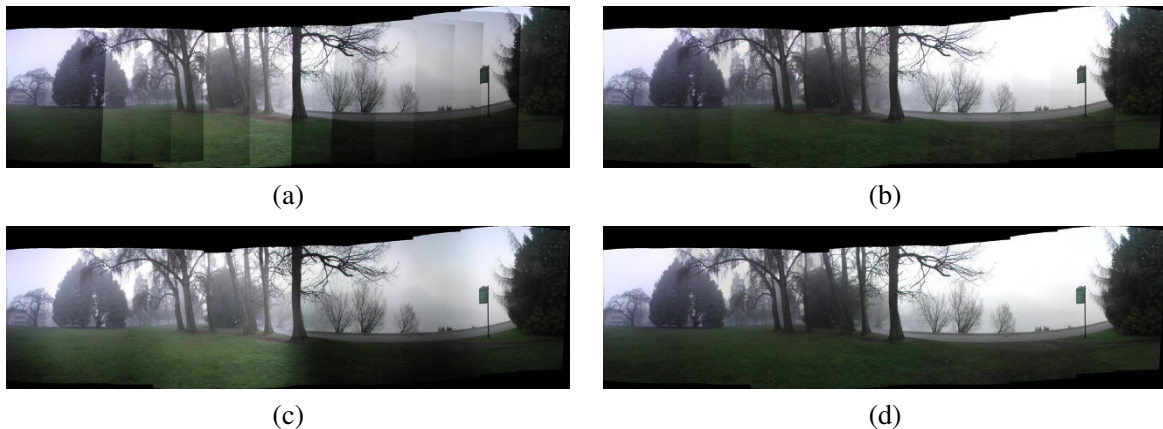
Figure 10.6 Simultaneous estimation of vignetting, exposure, and radiometric response (Goldman 2010) © 2011 IEEE: (a) original average of the input images; (b) after compensating for vignetting; (c) using gradient domain blending only (note the remaining mottled look); (d) after both vignetting compensation and blending.
