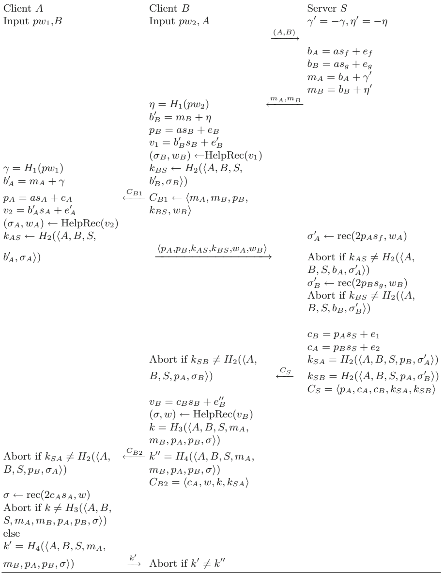
Fig. 1. Three-party password authenticated protocol: RLWE-3PAK, where s_S, e_S, s_f, e_f, s_g, e_g, s_B, e_B, e'_B, e''_B, e_A, e'_A, e_1, e_2 is sampled from \chi_\beta . Shared session key is sk = H_5(\langle A, B, S, m_A, m_B, p_A, p_B, \sigma \rangle) .
