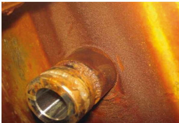
Fig. 6.6 Crevice corrosion of 317 L RO nozzles coupling high-pressure header to the RO membranes [52]
