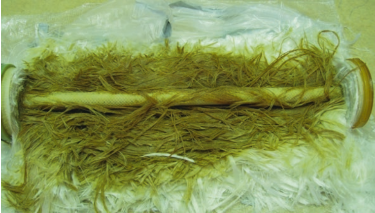
Fig. 3.7 Digital photographs of fouled HFF SWRO membrane
