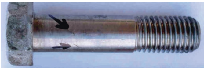
Fig. 5.17 MIC on seawater pump bolt in desalination intake
