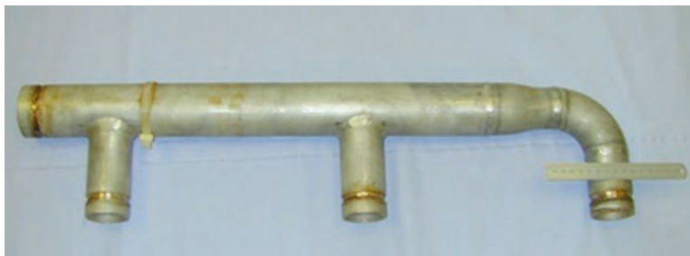
Fig. 6.8 Crevice corrosion of HP pipe spool made of Zeron 100® (Source: Rolled Alloys) [54]
