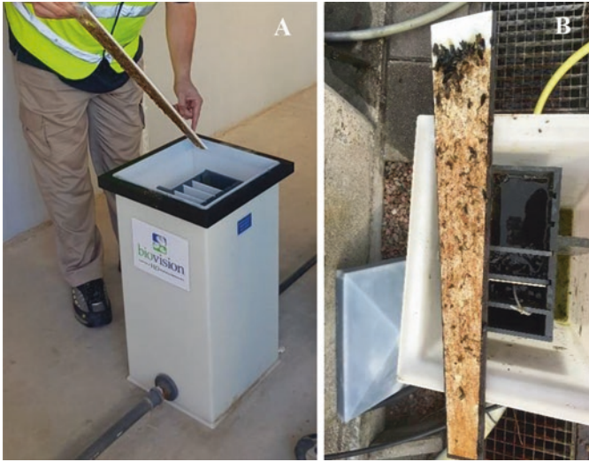
Fig. 16.11 H2O biovision monitor™ (A); Fouled coupons with marine biofouling (B). (Source: H2O Biofouling Solutions B.V)
