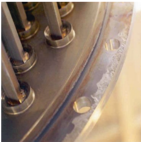
Fig. 6.6 Crevice corrosion of 317 L RO nozzles coupling high-pressure header to the RO membranes [52]
