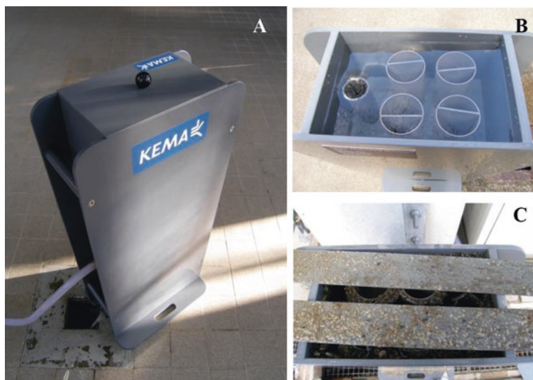
Fig. 16.10 KEMA biofouling monitor (A); Top view with the four fouling coupons (B); Fouled coupons with marine biofouling (C). (Source: KEMA Nederland B.V)
