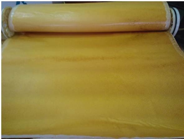
Fig. 3.8 Digital photographs of fouled spiral wound SWRO membrane
