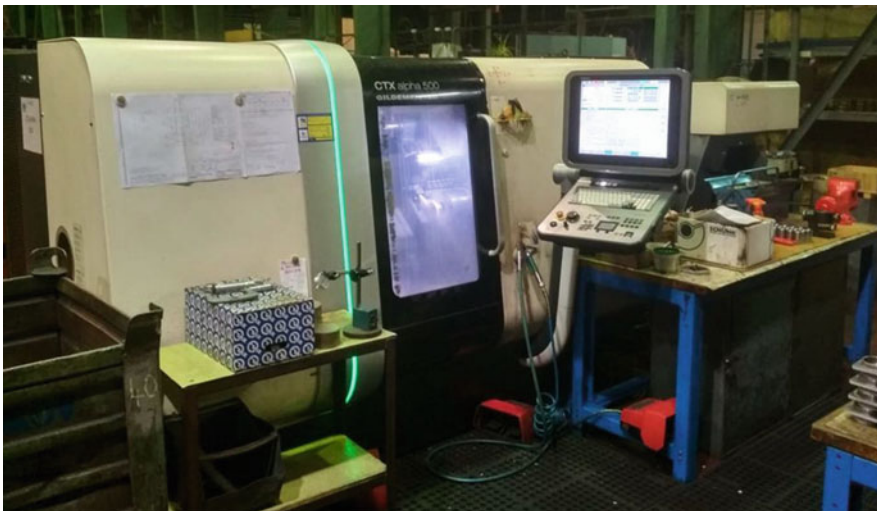
Fig. 7 Multi-axis double spindle turning CNC machining center CTX alpha 500
