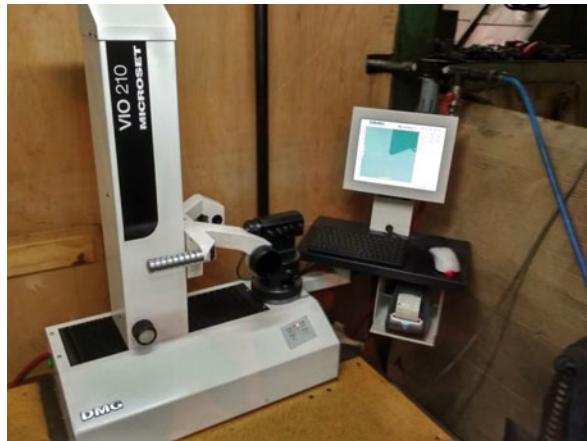
Fig. 10 The adjusting device DMG VIO 210 MICROSET
