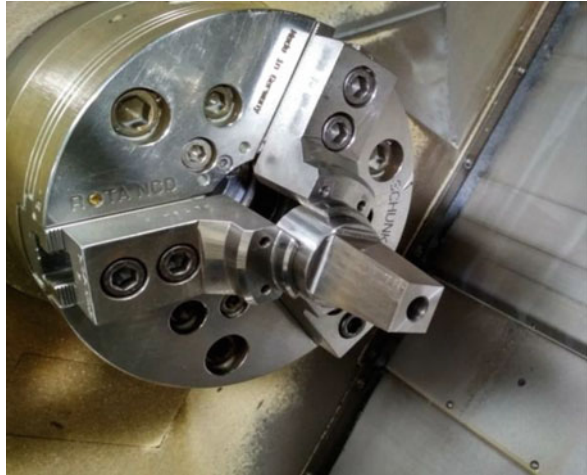
Fig. 11 Clamping component in the left chuck
