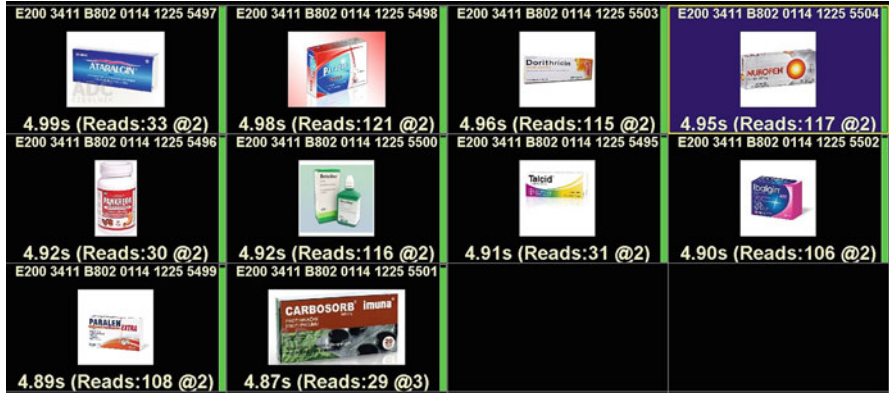
Fig. 5 Detection of RFID tags in a plastic box
