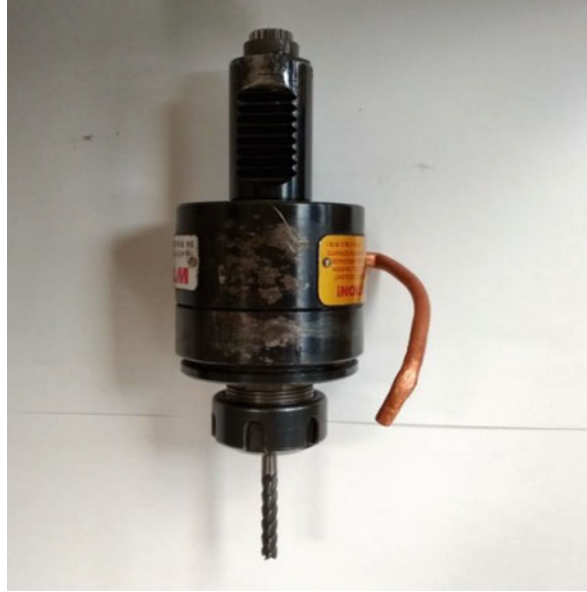
Fig. 9 Fig. 9. Finishing milling DORMER Product Selector S717 Ø6
