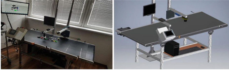
Fig. 5 Experimental quality control system (left) 3D model of device (right)
