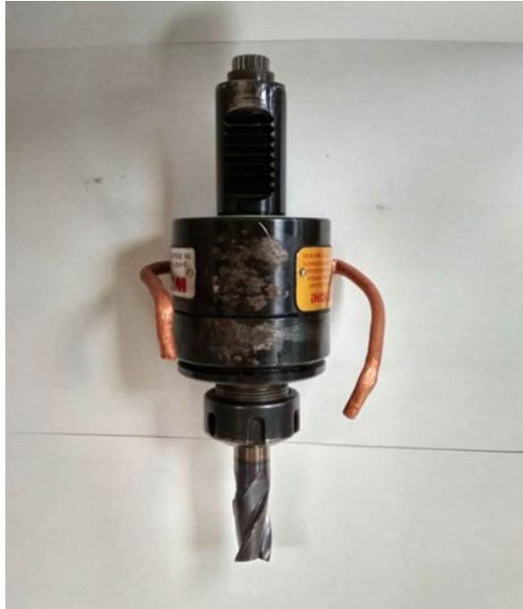
Fig. 8 Roughing milling tool DORMER S944 16.00 HM titanium aluminum nitride (TiAlN)
