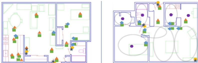
Fig. 2. Example of heterogeneous sensor layouts in the smart homes used to collect hh101 (left) and hh103 (right). Different shapes represent different sensor types.
