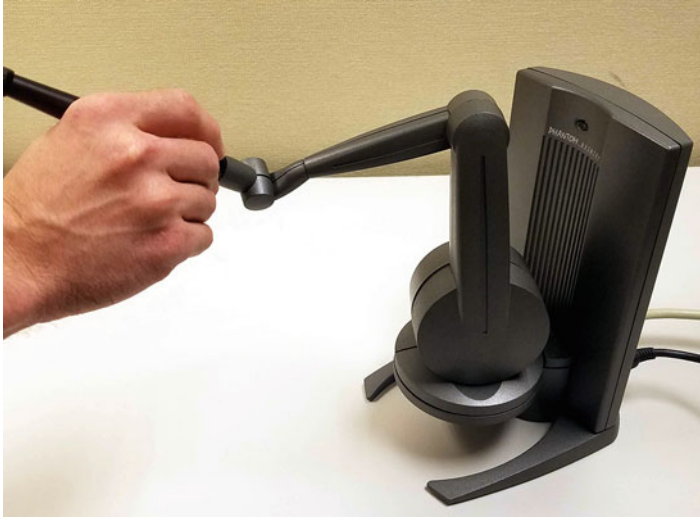
Fig. 4.6 Sensable Inc's PHANTOM Desktop, a force feedback device for haptic applications
