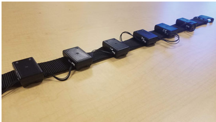
Fig. 4.8 Haptic Belt developed at the CUBiC Lab at Arizona State University [67]. The belt was designed to be modular and can be extended to fit more or fewer tactors connected in series. The location of the tactors can also be modified by simply sliding them along the belt
