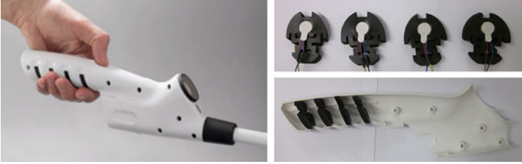
Fig. 2.3 Eyecane handle (left) and vibrotactile actuators mounted into cane handle (right). Each ERM is placed in the middle of a rubber ring (top right). A portion of the rings protrudes outward, where the fingers contact it on the surface (right bottom)
