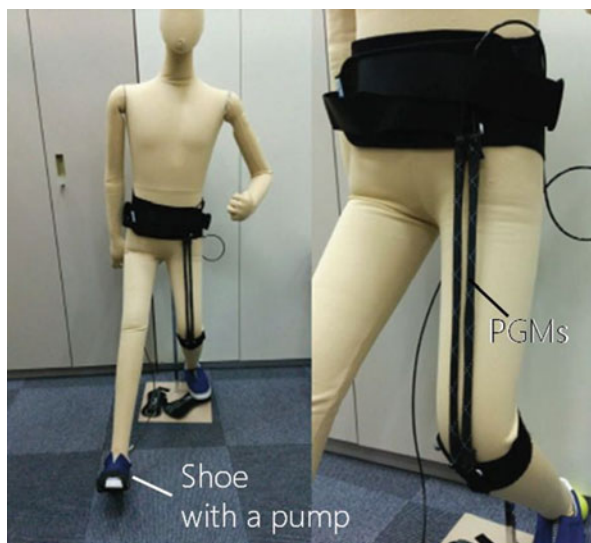
Fig. 8.4 Developed prototype of Unplugged Powered Suit
