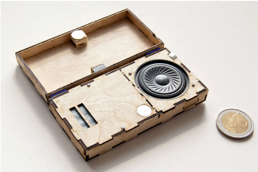
Fig. 1.3 The Audio Box was able to record and play back one single audio recording. It could also function as a container for small and haptically appealing objects
