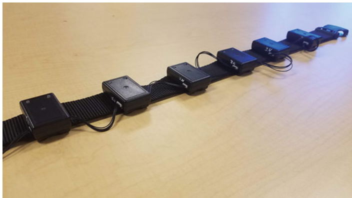
Fig. 4.8 Haptic Belt developed at the CUBiC Lab at Arizona State University [67]. The belt was designed to be modular and can be extended to fit more or fewer tactors connected in series. The location of the tactors can also be modified by simply sliding them along the belt
