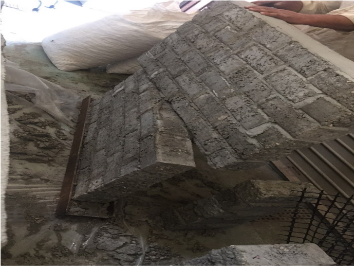
Fig. 3. One of the out-of-plane tested 7.5% slurry samples.
