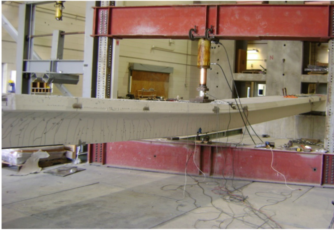
Fig. 10. BDT1 flexure test, final deflected shape
