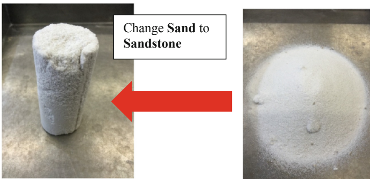
Fig. 1. EICP technique to convert sand to sandstone
