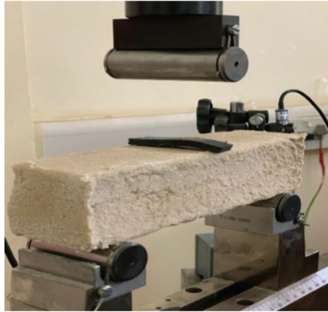
Fig. 5. Treated soil specimen during flexural test
