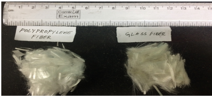
Fig. 2. Particle Image showing discrete polypropylene and glass fiber
