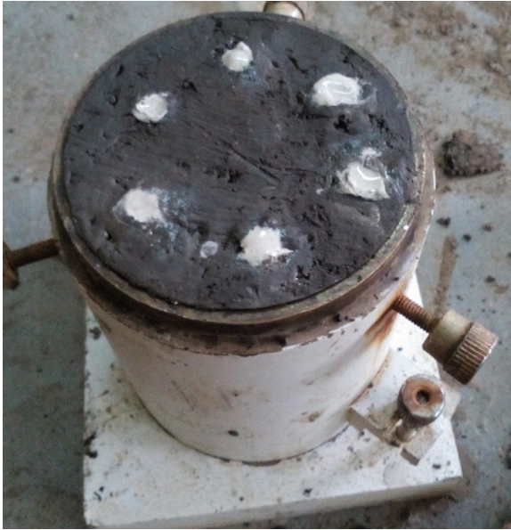
Fig. 1. 6 mm diameter columns grouted with industrial waste slurry in swell pressure mould
