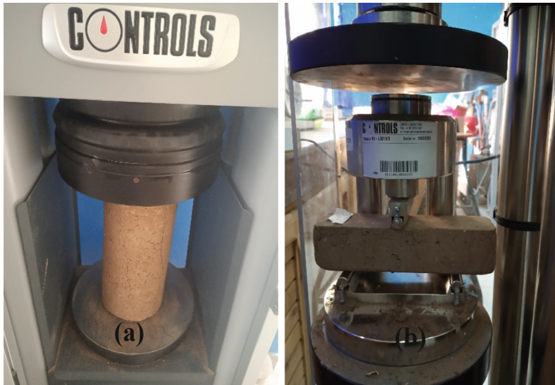
Fig. 2. (a) Compressive test (b) Three-point bending test
