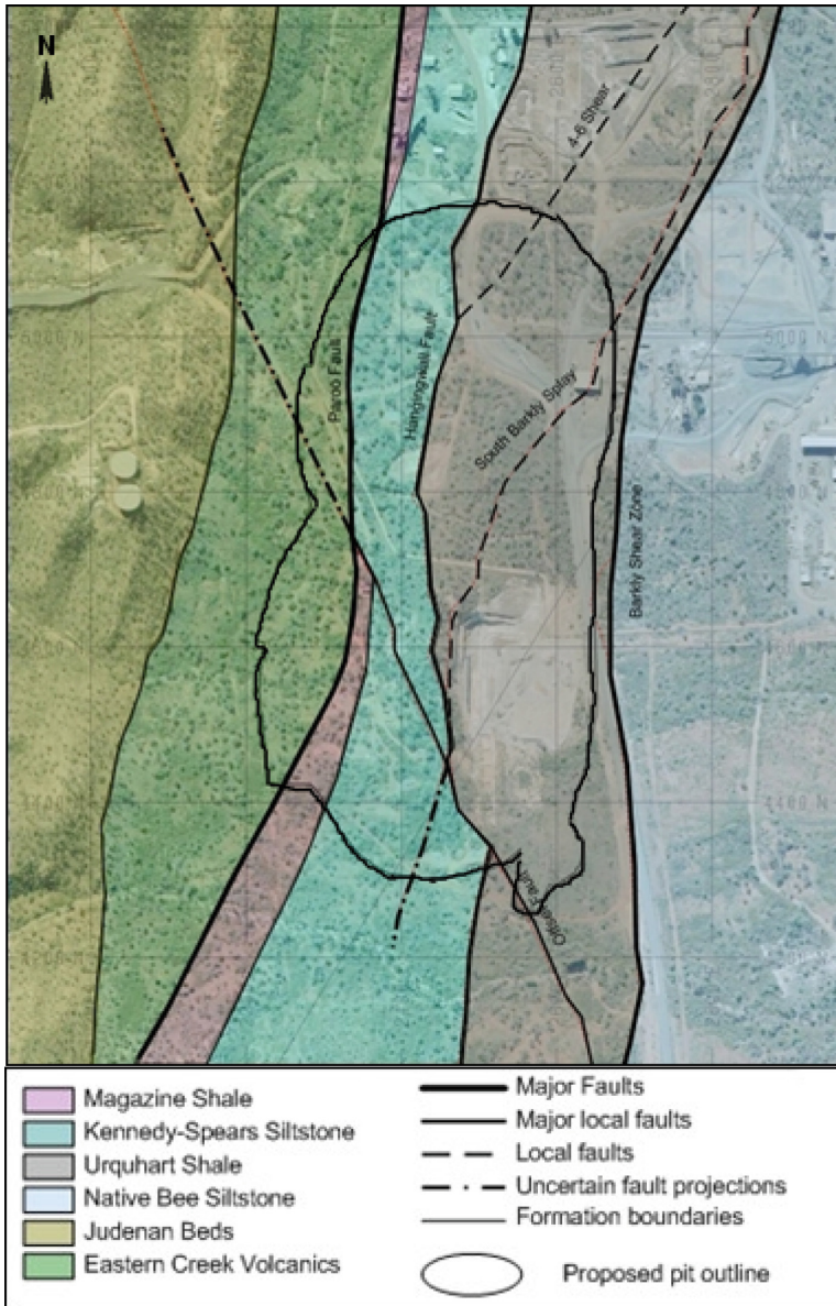
Fig. 4. Lithological domains intersecting Handlebar Hill open pit (after HH feasibility study 2007)
