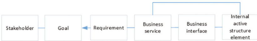
Fig. 1. Metamodel of ARMOR-Light with part of the metamodel of ArchiMate [7]. The lines represent many to many relations, the arrow represents a subset.
