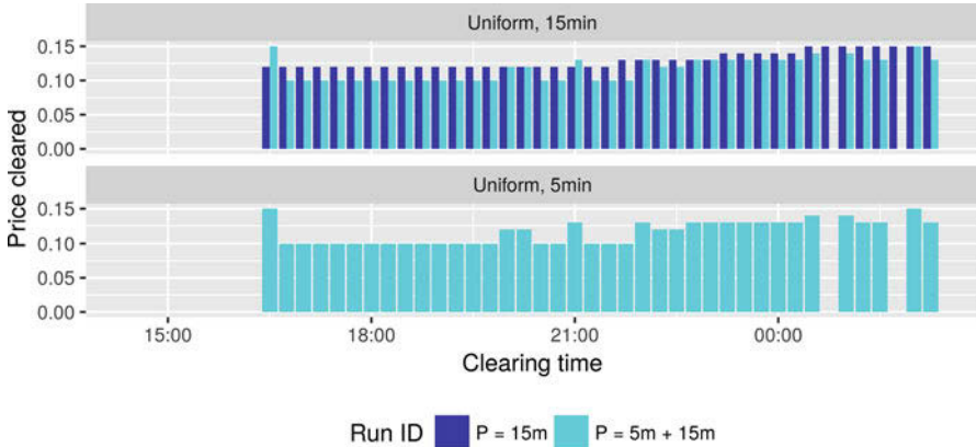
Fig. 21.3 Comparison of clearing price between a market with only one product (15 minutes delivery interval) and a market with two products (5 minutes and 15 minutes delivery time)
