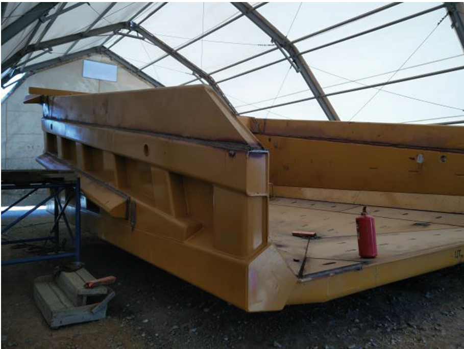
Fig. 3. Truck body with sideboards.
