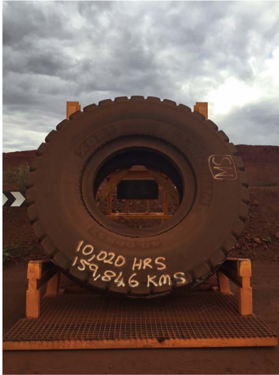
Fig. 3. AHT tyre at retirement (Price 2017)
