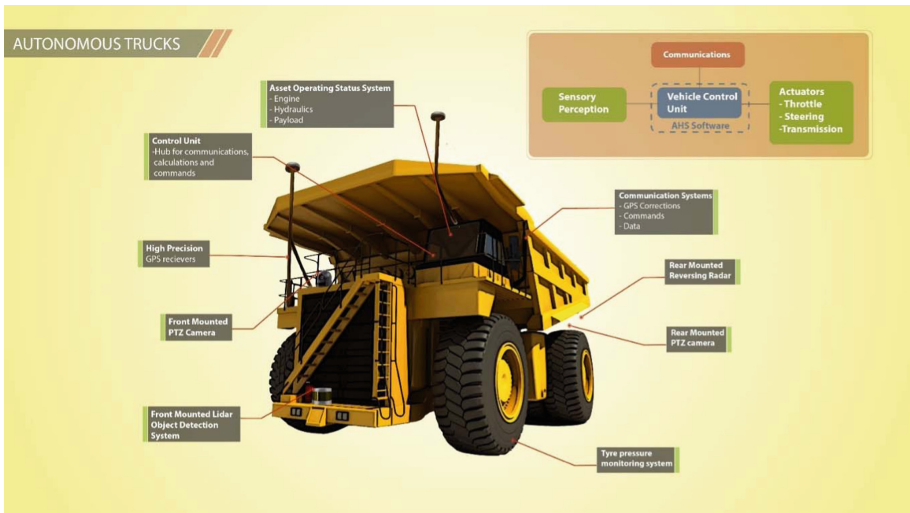
Fig. 1. Generic AHT onboard AHS equipment (Miller 2016).
