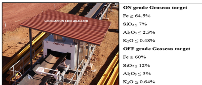
Fig. 5. Geoscan and the targets required to be measured by the geoscan
