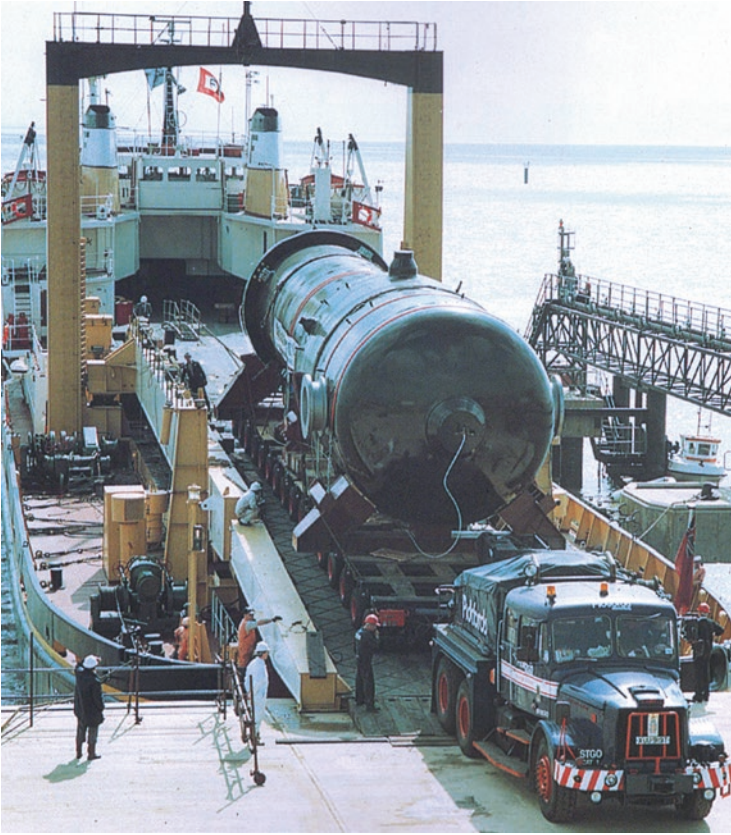
Fig. 6.6 Delivery of a PWR steam generator
