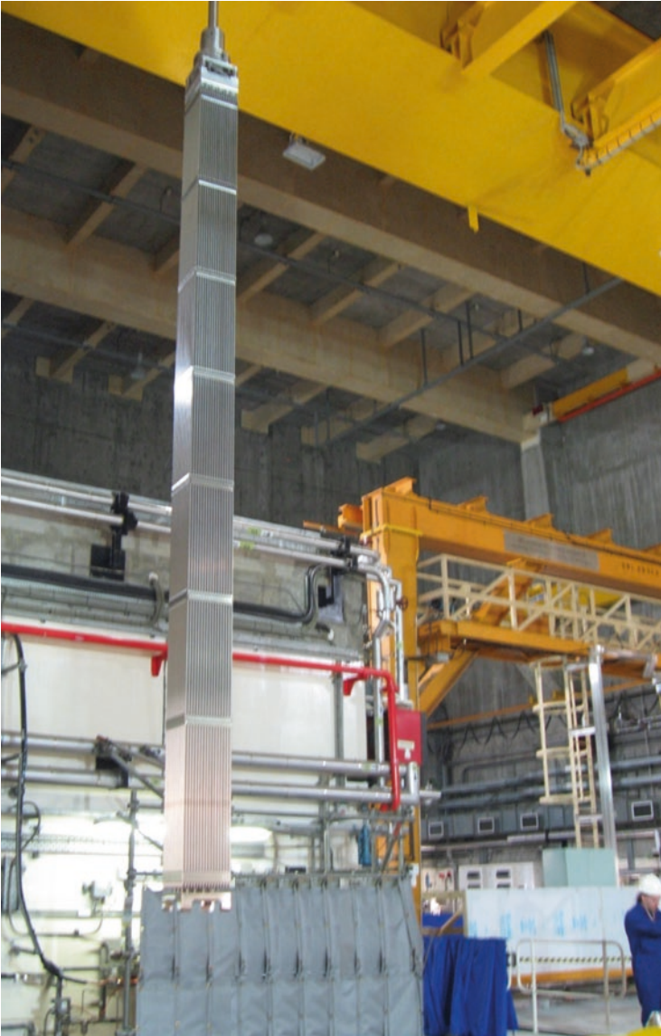
Fig. 3.2 A PWR fuel assembly
