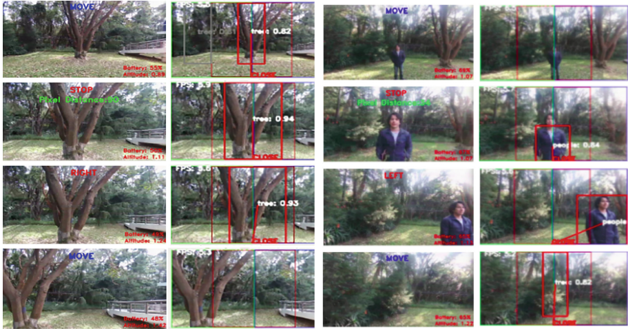
Fig. 6. Tree and people detection and collision avoidance in a real environment with one obstacle during autonomous flight
