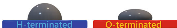
Fig. 3 Scheme illustrating the different contact angles observed in hydrogenated (left) and O -terminated (right) BDD surfaces
