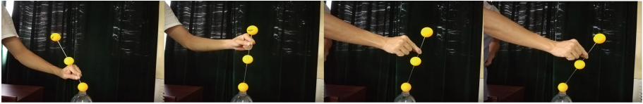
Fig. 3. Sample images of a 1D object used for camera calibration.
