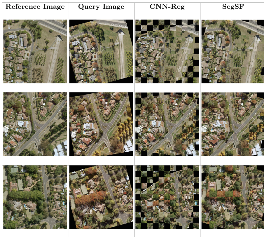
Fig. 2. Checkerboard results of registering multitemporal images using CNN-Reg and SegSF
