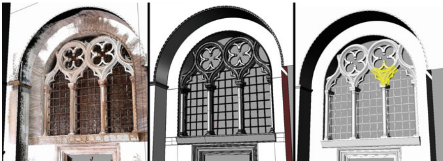
Fig. 1 Example of modelling by NURBS. From the left: pointcloud, geometric model and final result with a single element highlighted. Source He.Su.Tech. group
