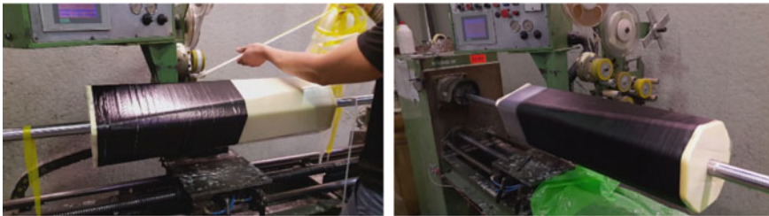
Fig. 4 Filament winding of the mold with carbon fibers
