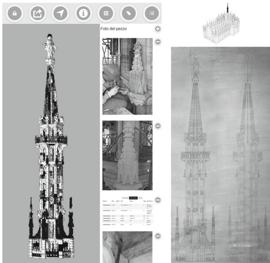
Fig. 2 On the left, a detail of the final part of the Main Spire visualized on the online system. The blocks subject to intervention (different colors according to the type of intervention) with some example images are provided; on the right the same detail in the original drawing made by Veneranda Fabbrica, on 1:20 scale, January 7, 1941
