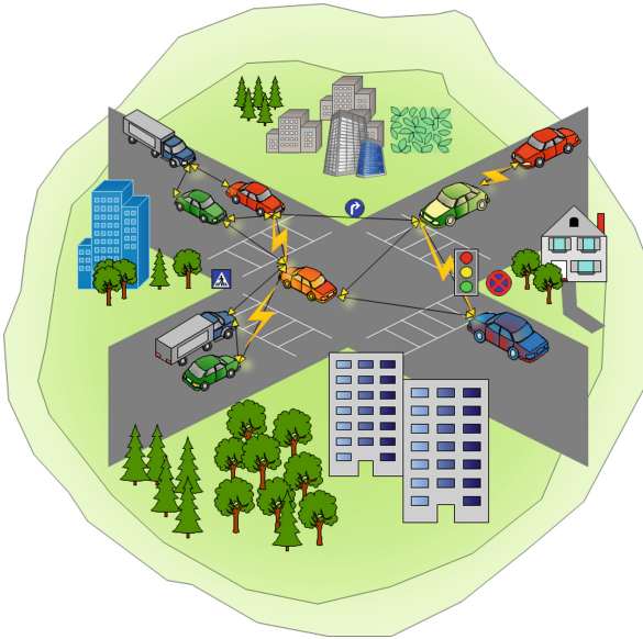
Fig. 2. Diagram of a sample connected smart vehicular network.
