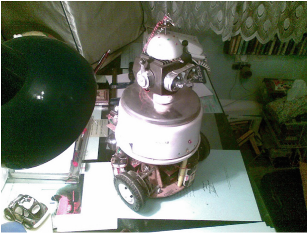
Fig. 1. First Iranian pedagogic Robot called “PARS-1B”, with AI Graph Search Algorithm to track and find barriers and targets. Developed by Author, in Sharif University of Technology, E.E. Dept, year 1986.
