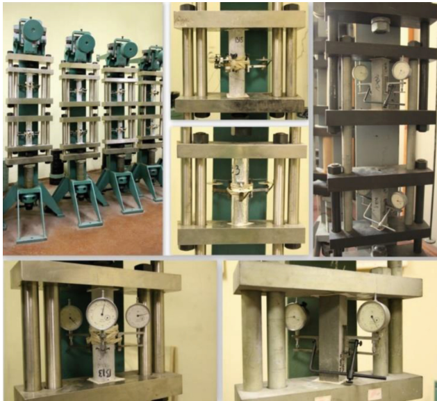
Fig. 2. Determination of uniaxial compressive creep strains with the creep lever test stands (RTU lab).
