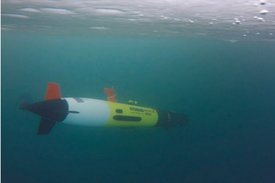
Fig. 9.6 AUV launched under sea ice. The under-ice environment is normally dark as for the Polar Night operations in open waters
