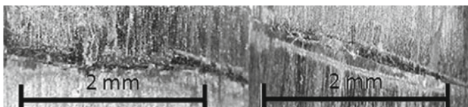
Fig. 4 Specimens with carbon fibers; damage to the fibers in the location of the action of test equipment
