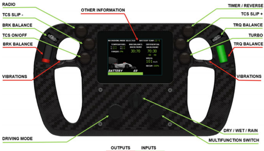
Fig. 1 Control and information elements layout according to ergonomic rules
