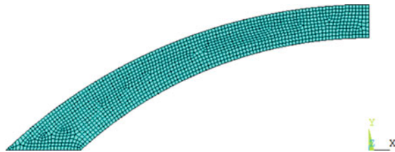
Fig. 5 FEM model of cornea
