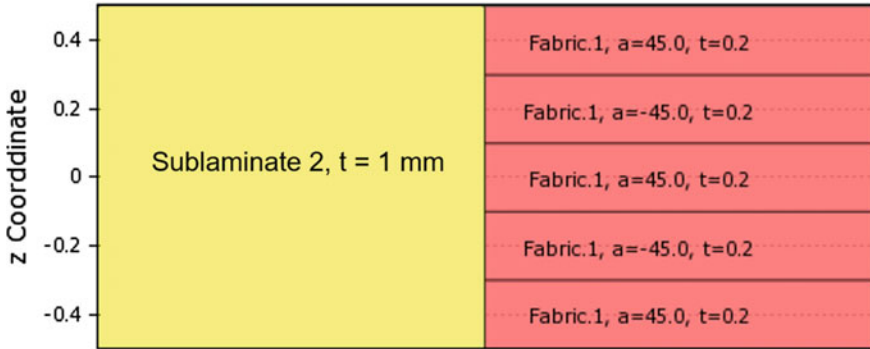
Fig. 2 Angle direction of layers for second set
