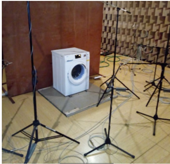
Fig. 1 Position of the washing machine within the anechoic chamber
