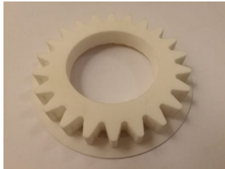
Fig. 6 Sprocket made by SLS method
