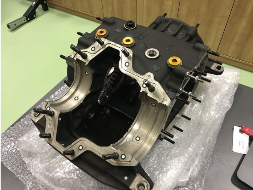
Fig. 1 Gearbox case with damaged bearing housings. Prepared to be scanned
