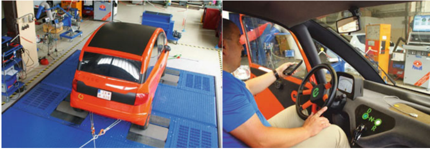
Fig. 5 Electric car Edison on the roller dynamometer MAHA
