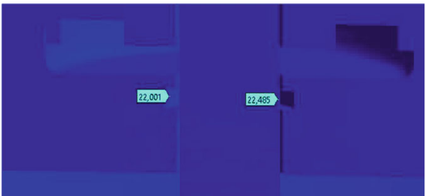
Fig. 7 Temperatures in locations of contact between the seals and working components—blank holder
