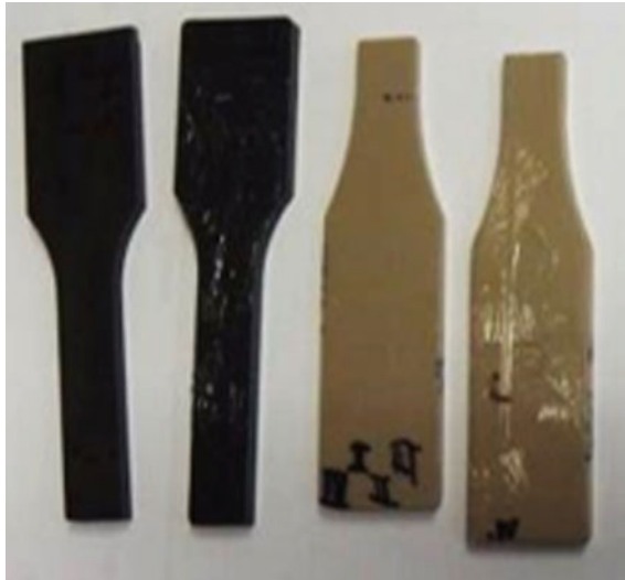
Fig. 1 Photograph of real experimental specimens, left side: composite material with carbon fiber, and right side: composite material with glass fiber
