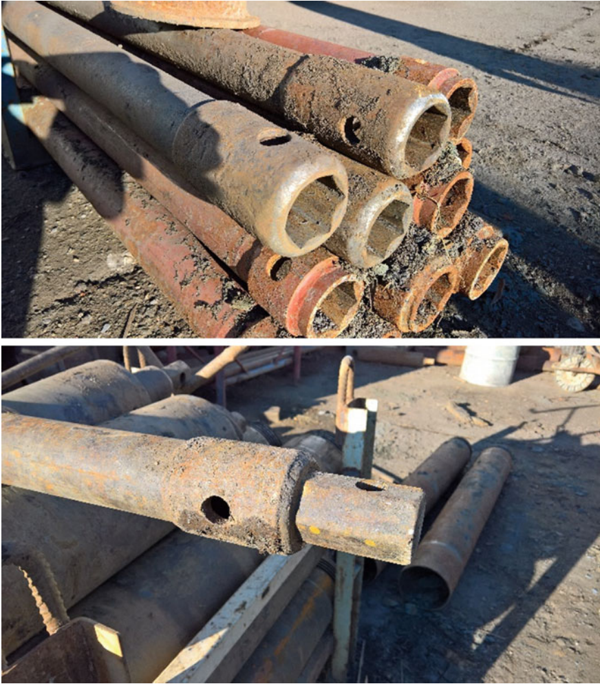
Fig. 2 Drilling rods—connection by means of the inner and outer hexagon
