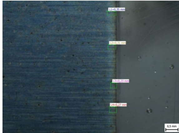
Fig. 3 Cross section of 100Cr6 sample with depth of the nitride layer (etched with 3% Nital)
