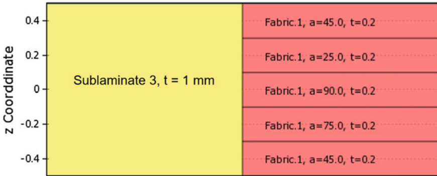
Fig. 3 Angle direction of layers for third set
