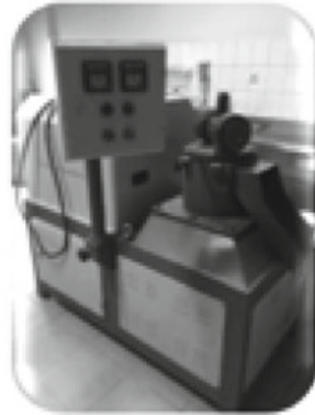
Fig. 1 Manually fed laboratory-type pelleting machine with horizontal rotating matrix
