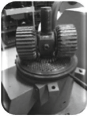
Fig. 1 Manually fed laboratory-type pelleting machine with horizontal rotating matrix
