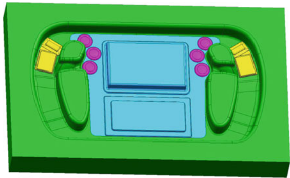
Fig. 4 The shape for laminating the front half of the steering wheel on which the blue, yellow, and pink colors are marked by the interchangeable runners
