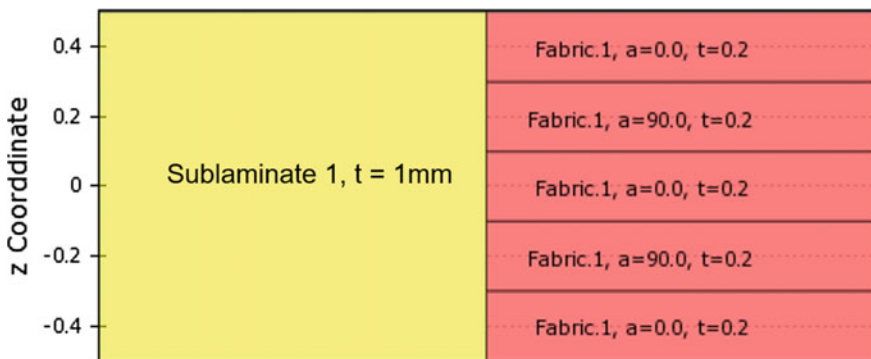
Fig. 1 Angle direction of layers for first set
