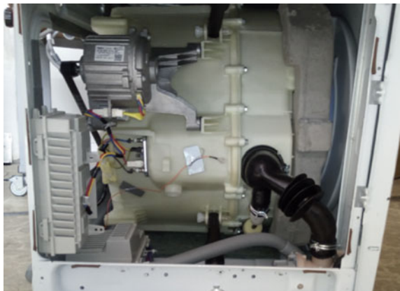
Fig. 4 Sensor placement on the drum assembly
