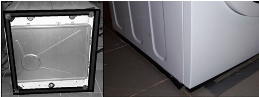
Fig. 8 Placement of the acoustic insulation at the bottom part of the washing machine
