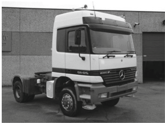
Fig. 1 MERCEDES-BENZ ACTROS 2040, 4 × 4 tractor
