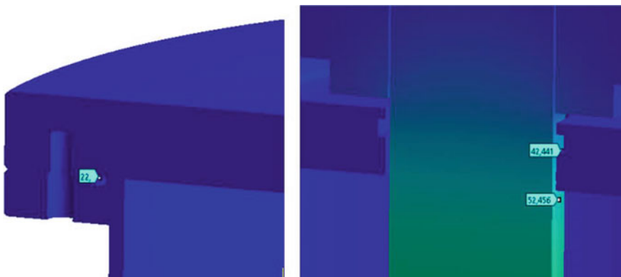
Fig. 5 Temperatures in locations of contact between the seals and working components—vacuum chamber and punch
