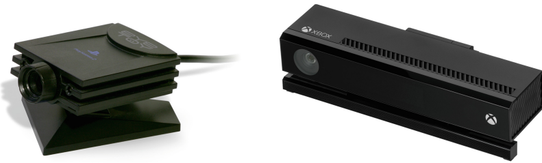
Fig. 8. Computer vision devices: Sony EyeToy (left) and Microsoft Kinect (right).
