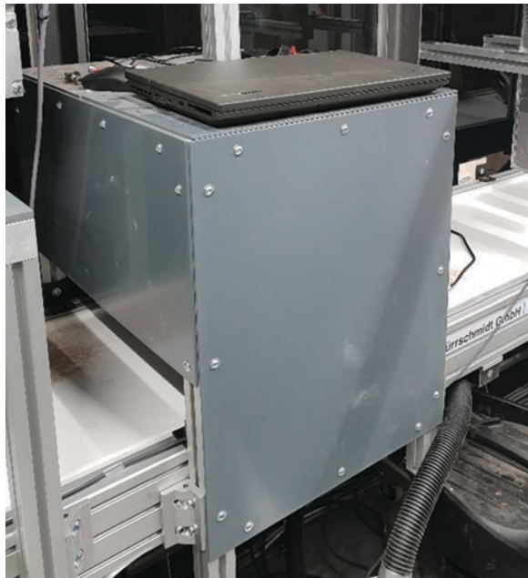
Fig. 8.6 Darkened room over the assembly line with industrial camera inside
