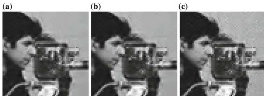
Fig. 3 Cameraman test problem blown-ups of the reconstructions obtained with different methods: a NMLBA-Str, b NMLBA, c FISTA
