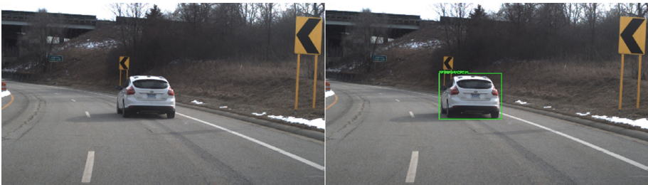
Fig. 5. Original input image (left), output of object detection algorithm with a marked bounding box along with the probability of prediction (right)
