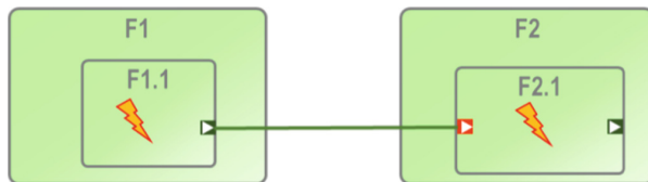
Fig. 2. MBSA modeling of functional architecture. Thunderbolts represent failure modes that are modeled inside functions.
