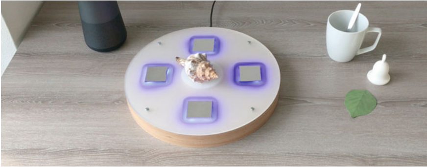
Fig. 13.2 The dementia soundboard served as a tangible means for playing soundscapes by placing the corresponding objects on the central circle. By tapping the surrounding touchpads, the sound layers that make up the soundscape could be muted or unmuted
