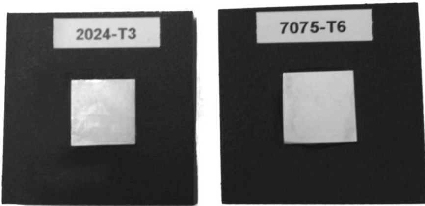
Fig. 5.26 Two 1.0" × 1.0" AA 2024-T3 and AA 7074-T6 panels prepared for microscopic analysis
