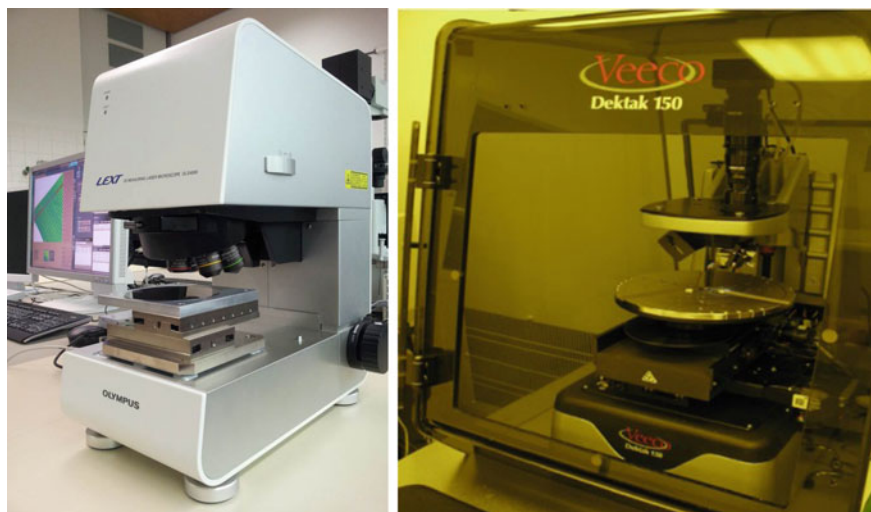
Fig. 5.8 Left: LEXT OLS4000 3D Laser Measuring Microscope. Right: Bruker's Dektak ® Stylus Profiler
