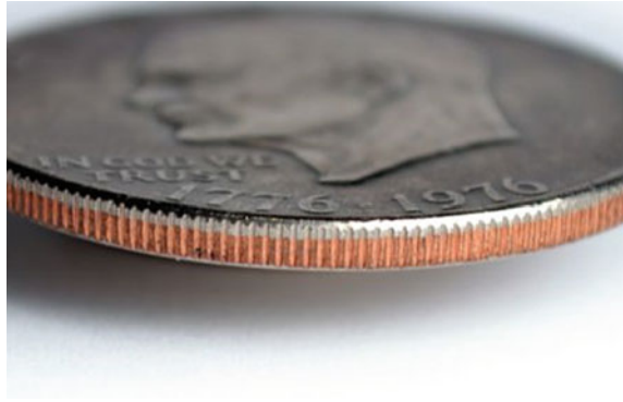
Fig. 4.3 US coin clad with copper and nickel
