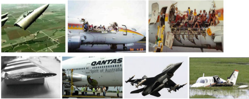
Fig. 7.3 Catastrophic effects of corrosion and cracking
