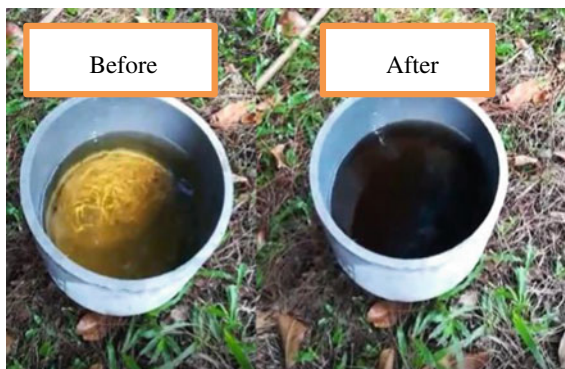
Fig. 3 This is the reaction of the groundwater after 40 s exposed to the oxygen
