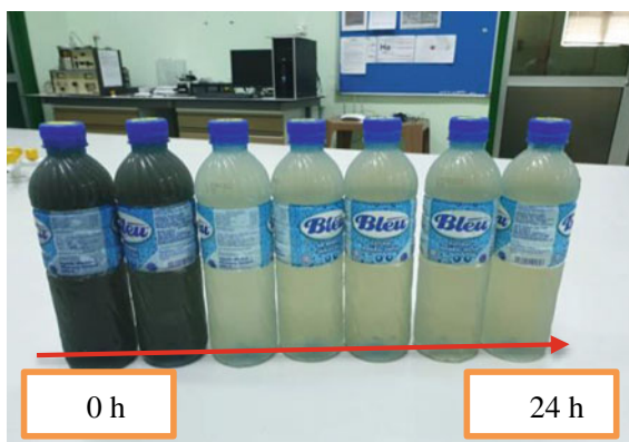
Fig. 4 This is the reaction of the groundwater after 24 h exposed to the oxygen
