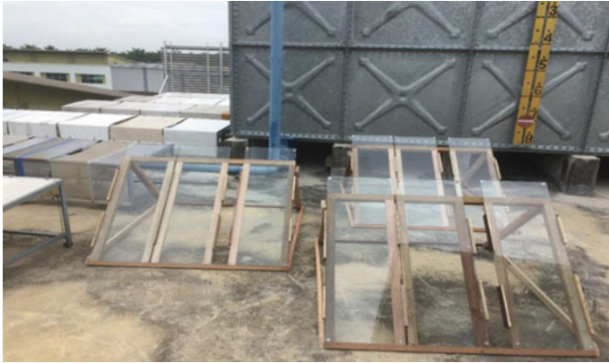
Fig. 1 Setup of glass samples for direct exposure
