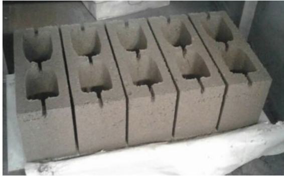
Fig. 7 Self-standing GHB4 before oven curing—immediately after casting
