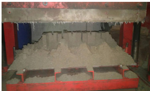
Fig. 6 Collapse of GHB2
