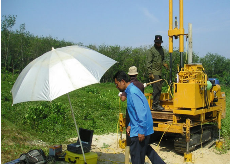
Fig. 2 CPTU assembly of the School of Civil Engineering, Universiti Sains Malaysia consisting of crawler mounted Hyson 100 kN penetration system and Vertek-Hogentogler data acquisition system
