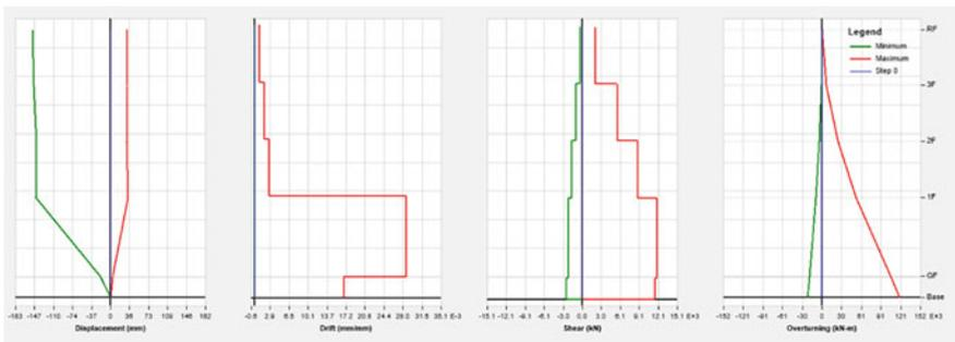
Fig. 6 Structural response in x-axis of building in Lahad Datu under earthquake scenario 2
