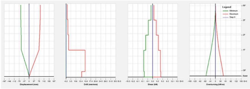
Fig. 2 Structural response in x-axis of building in Ranau under earthquake scenario 1
