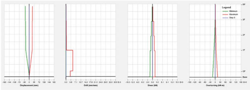
Fig. 11 Structural response in y-axis of building in Kota Kinabalu under earthquake scenario 3
