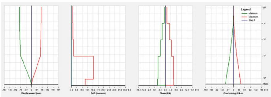
Fig. 3 Structural response in y-axis of building in Ranau under earthquake scenario 1
