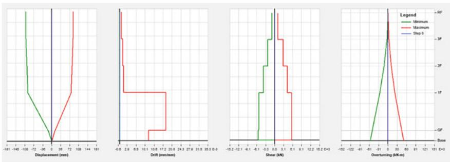
Fig. 9 Structural response in y-axis of building in Ranau under earthquake scenario 3
