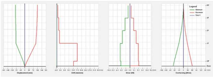
Fig. 8 Structural response in x-axis of building in Ranau under earthquake scenario 3
