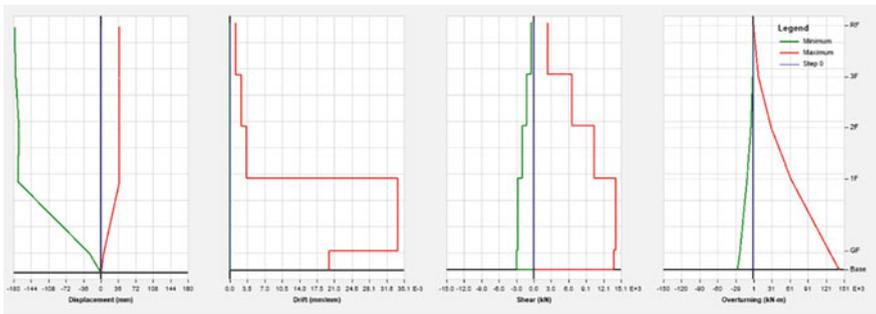
Fig. 12 Structural response in x-axis of building in Lahad Datu under earthquake scenario 4
