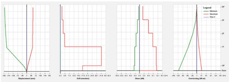
Fig. 13 Structural response in y-axis of building in Lahad Datu under earthquake scenario 4
