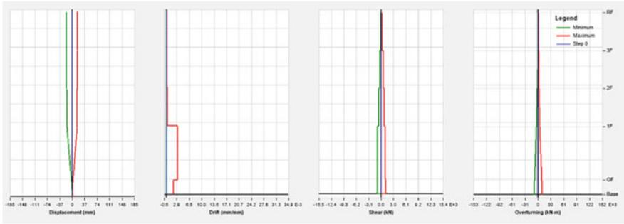
Fig. 5 Structural response in y-axis of building in Kota Kinabalu under earthquake scenario 1
