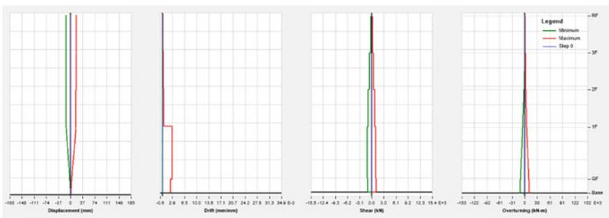
Fig. 4 Structural response in x-axis of building in Kota Kinabalu under earthquake scenario 1
