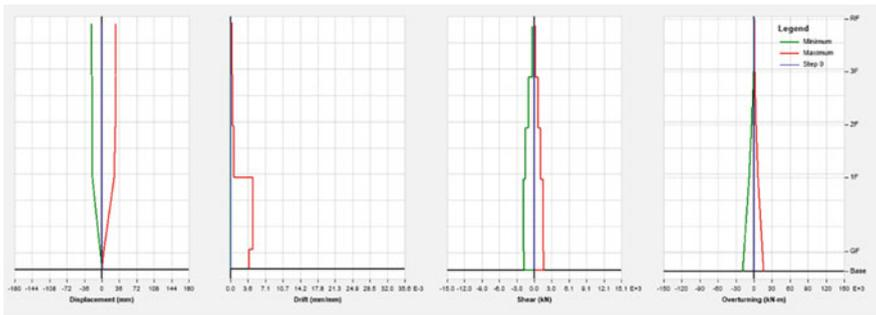
Fig. 10 Structural response in x-axis of building in Kota Kinabalu under earthquake scenario 3
