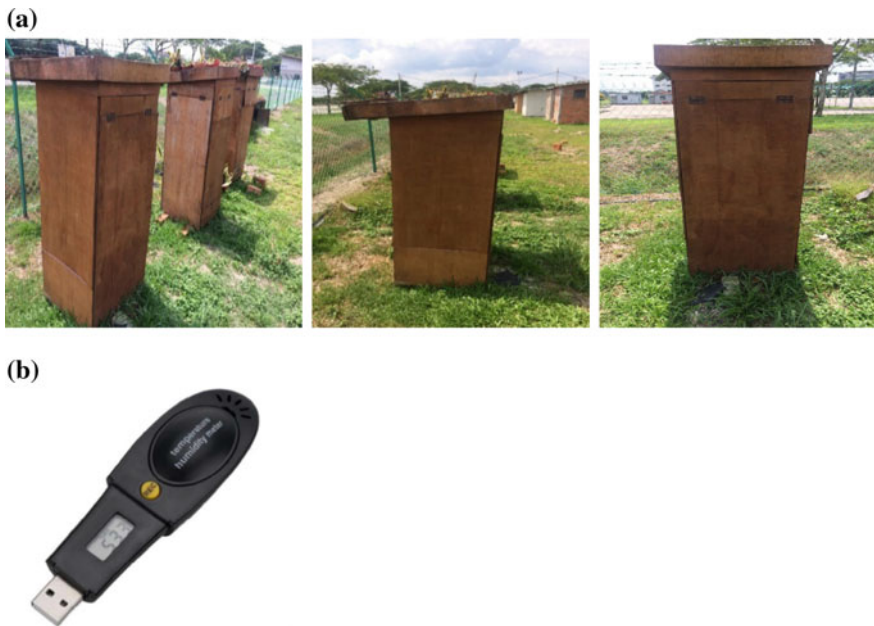
Fig. 1 a Small-scale roof houses, b USB hygrometer data logger
