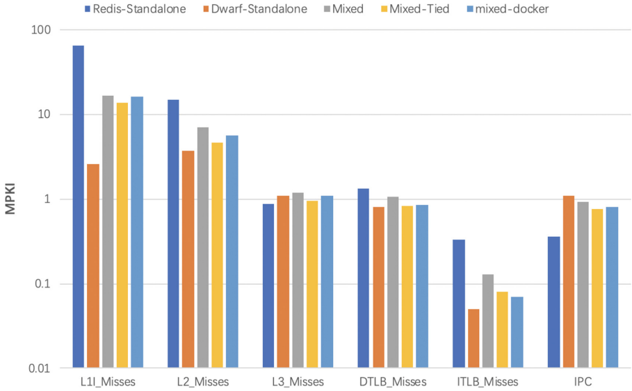
Fig. 6. The architecture metrics of the server node
