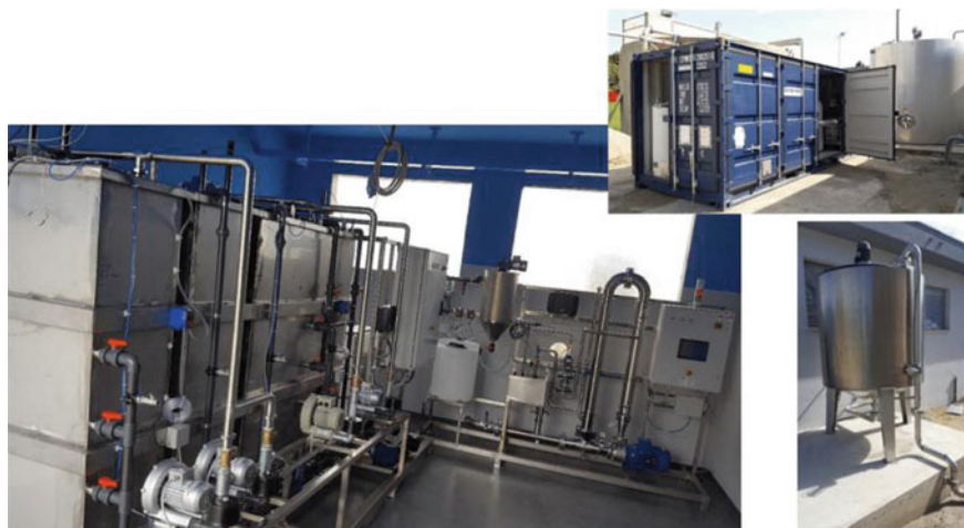
Fig. 5 Carbonera-Smartech 5-PHA and Struvite Recovery from anaerobic supernatants-years 2016 SMART-Plant Project ( www.smart-plant.eu )—Coordinator Università Politecnica delle Marche; Referent Partner University of Verona
