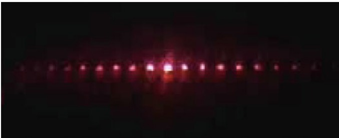
Fig. 5 Transient grating diffraction pattern due to colossal nonlinearity of dye-doped nematic liquid crystals (Reprinted with permission from ref. [48], Optical Society of America)
