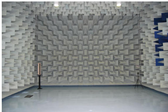
Fig. 1 Semianechoic chamber at the department of information engineering used for audio experiments
