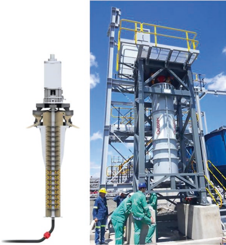
Fig. 4.8 Outotec industrial HIGmill (Letho et al. 2013)
