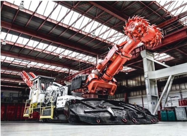
Fig. 3.1 Sandvik cutting machine, Roadheader MR341 roadheader for mining (Sandvik Mining and Construction 2007)
