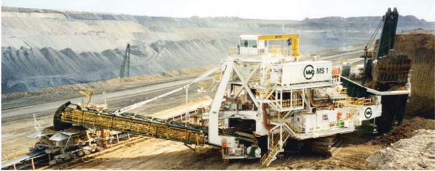
Fig. 3.11 Fully mobile sizer (Crusher) (Courtesy of MMD) (Johnson Marc 2014)
