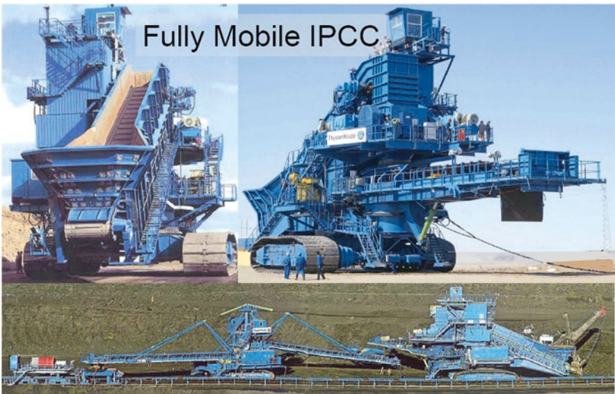
Fig. 3.10 Fully mobile IPCC (Koehler 2010)
