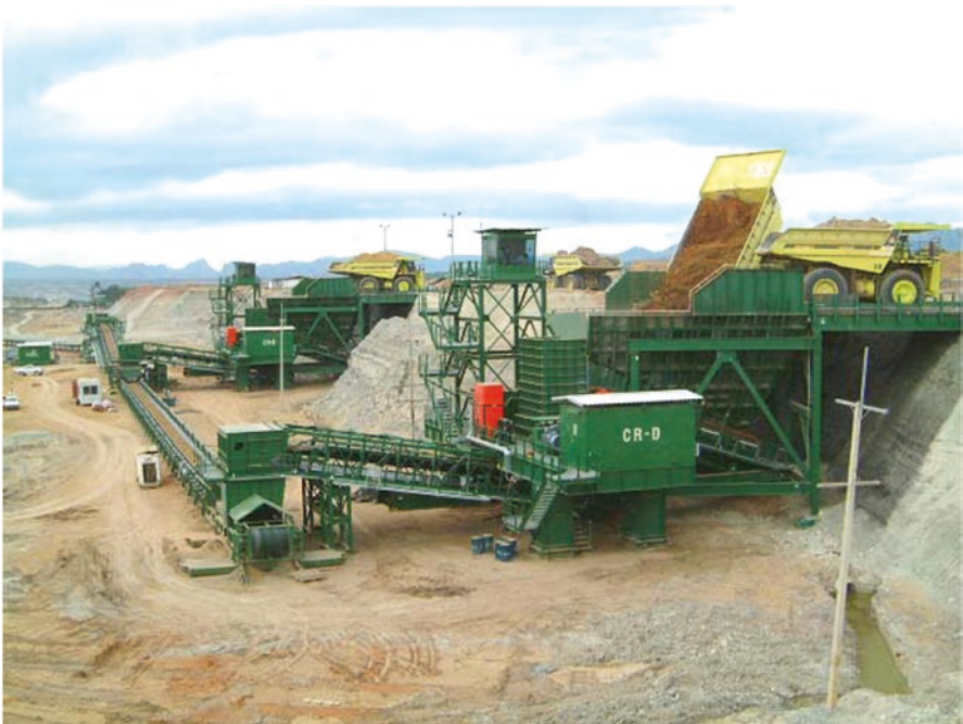
Fig. 3.8 Semi-mobile IPCC system (Cooper Allen 2010)
