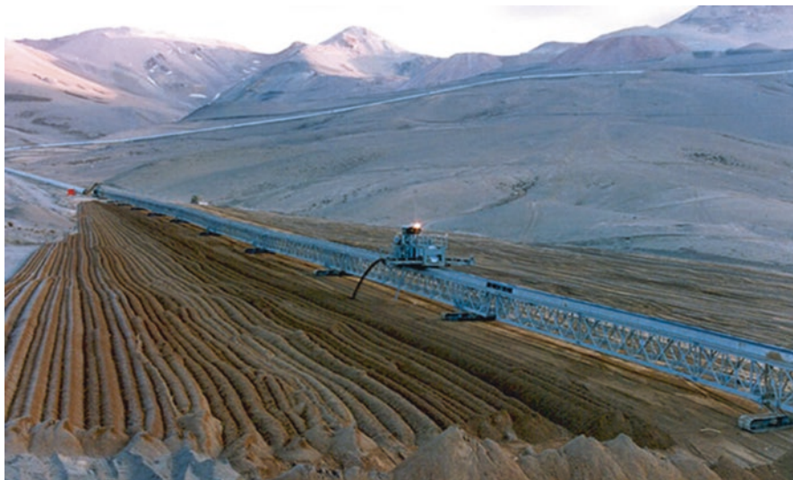
Fig. 11.3 Dry stacked tailings disposal La Coipa, Chile
